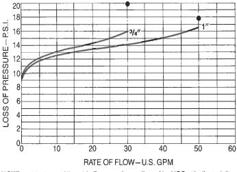
NOTE: • Maximum Allowable Pressure Loss allowed by USC at indicated flow.
